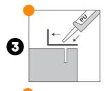
Insert plugs into holes and apply structural adhesive (e.g.CA290 adhesive) to the underside of stair nosing profile (1 to 2 beads in a straight line to the riser edge and beside screw holes along the entire length) to cushion any step variance and to prevent the nosing from rocking.
